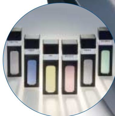
Certified test filters and simple menu-guided quality assurance in accordance with GLP.
